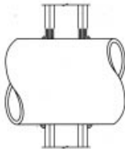
3M FireDam 150+ Caulk used in applications where metal pipe penetrates through gypsum board. UL System W-L-1167.
